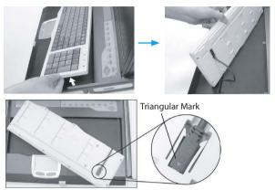
**NOTE:** There is a round hole under the drawer, which can be used to pass one finger through allowing for easier removal of the keyboard (pushing upwards). The triangular mark on the mini USB connector must face outwards.
